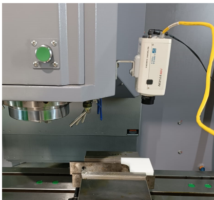
Figure 14. Part setup on HAAS VF1 milling machine
