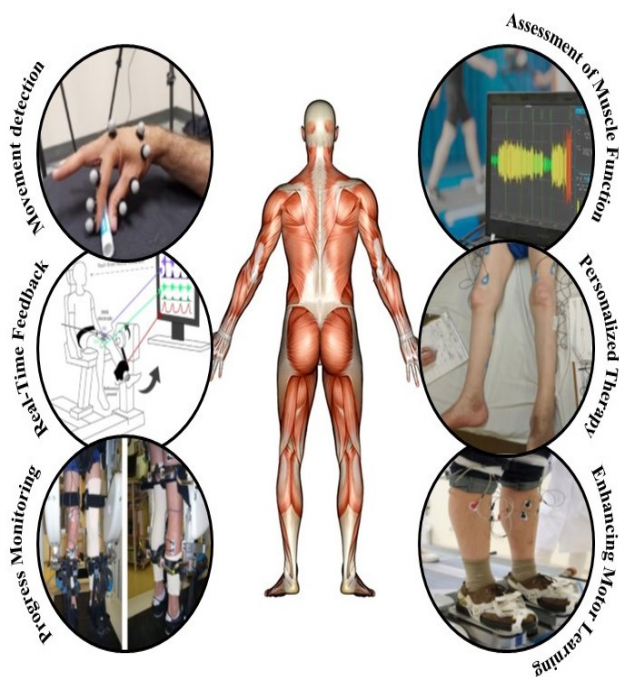
Figure 5. Role of EMG in Rehabilitation and Movement Detection: Rehabilitation methods, including physical, occupational, and robotic-assisted therapy, restore function. Movement detection uses tools like motion capture, wearable sensors, and EMG to monitor motor function
