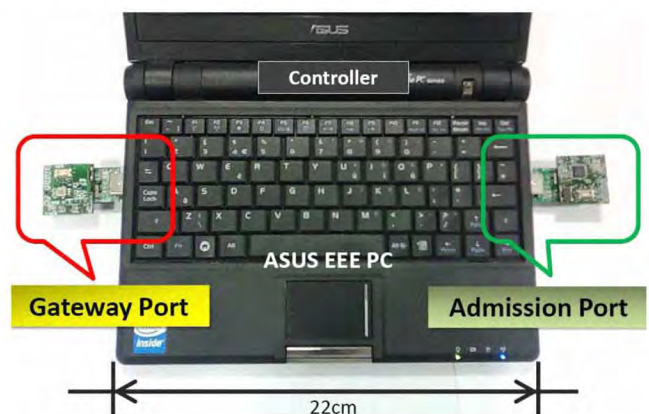
Figure 5. The prototype of a personal controller (ASUS EEE PC) that operates two USB sensor ports, one acting as a gateway to wireless biosensors and one as the secure physical channel of new sensor admission.
