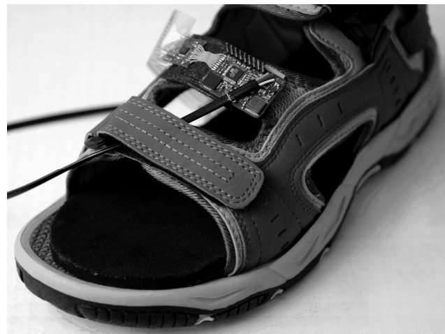
Figure 3 During test measurements, the capacitive insole sensor was placed in a sandal with read-out electronics.
