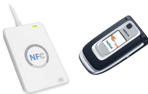
Fig. 7 There are several NFC readers available as– including the above ACR122 NFC Contactless Smart Card Reader (shown next to the Nokia 6131 NFC phone, used in this project)
