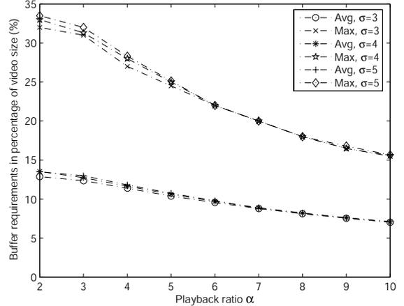
Figure 5: Comparison of required buffers of the HRAB normal case.
