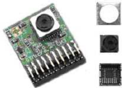
Figure 7: VS6724 single-chip camera module from ST microelectronics. The left picture shows the whole circuit board while the right picture shows the image sensor.
