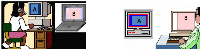
Figure 1. Distributed side-by-side interaction model. The display of the primary computer of the left (right) developer, A(B), is shown on the awareness computer of the right (left) developer.
