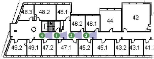
Figure 5: Linear camera setup in a hallway.
