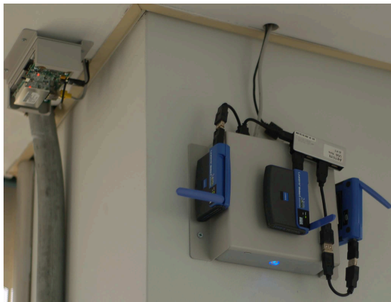
Fig. 2. Bottom right: WiSEMesh node deployment in the office building. Top left: Sensor network node.
