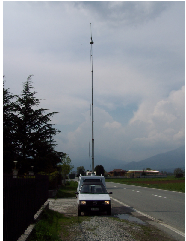
Figure 3. Equipped mobile vehicle with telescopic mast.
