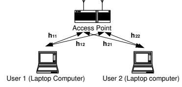
Fig. 2. The AP communicates simultaneously with two users over a single channel.
