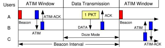
Fig. 1. Basic mechanism of IEEE 802.11 PSM.
