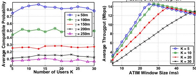
Fig. 5. (a) Compatible probability vs.  $K$ . (b) Throughput vs. ATIM window size.
