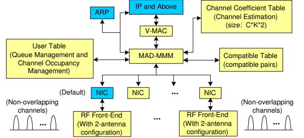
Fig. 3. MAC-OMA/MM firmware architecture in the AP.
