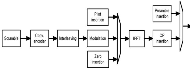
**Fig. 2.** Transmitter structure of IEEE802.11p physical layer
