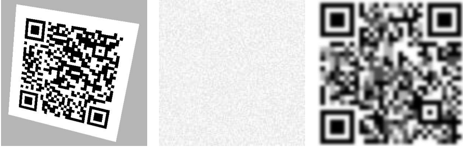
(a) Three degrees of freedom rotation of a QR Code (b) A white image containing 10% of random image noise (c) A DQR Code containing 10% of random image blur with \sigma = 0.3 matrix blocks
