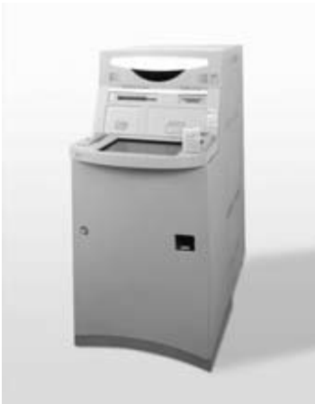
Fig. 1. ATM with palm vein pattern authentication sensor unit
