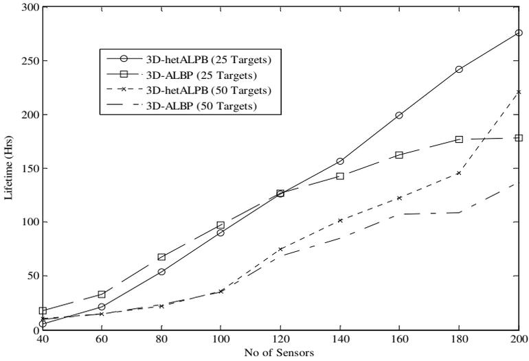
**Fig. 1.** Network lifetime with respect to number of sensors for linear energy model at 30M sensing range
