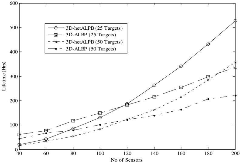
**Fig. 3.** Network lifetime with respect to number of sensors for linear energy model at 60M sensing range
