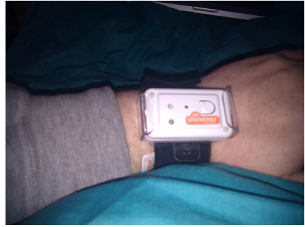
Fig. 6. Shimmer as a wearable sensor
