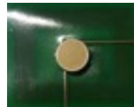
Fig. 4. RFID tag planar coil with the pressure sensor chip embedded in the middle
