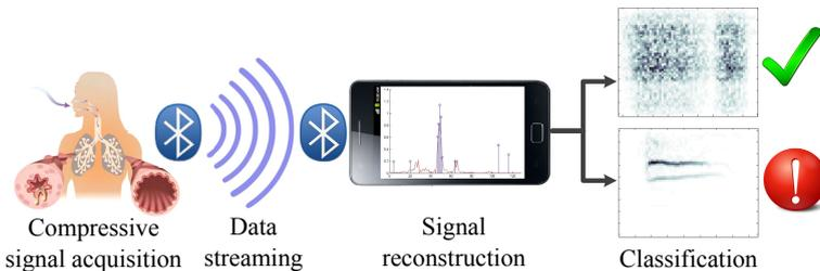
Fig. 1. Architecture of the asthma monitoring system
