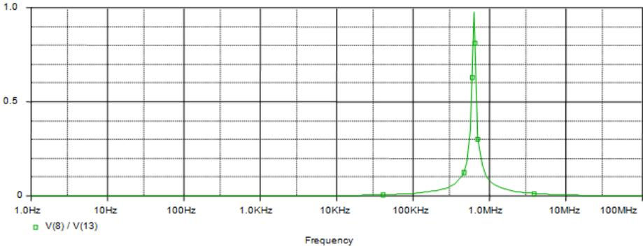
Fig. 8. Response of Second Order Resonance Section
