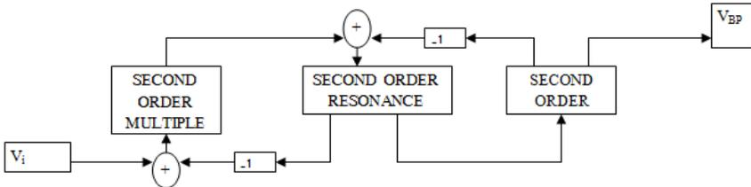
Fig. 6. Block Diagram of Sixth Order Leapfrog Filter (Bandpass Section)
