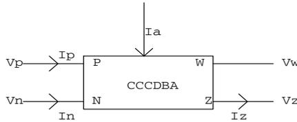
Fig. 1. Symbolic representation of current-controlled CDBA [7],[8]
