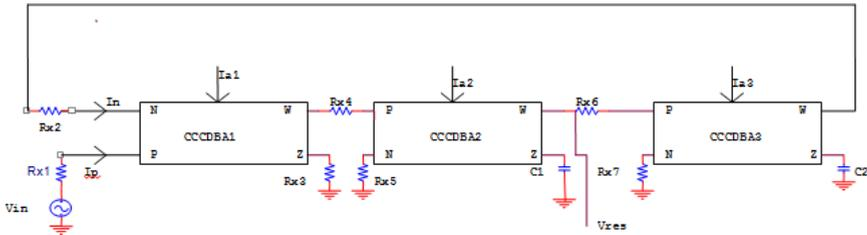
Fig. 5. Circuit Realization of Resonant Section Using CCCDBA
