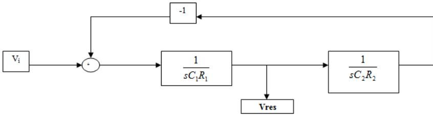
Fig. 4. Block Diagram of Resonant Section
