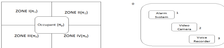
Fig. 1a. Smart Home as Distributed P System Fig. 1b. The P System representing a zone
