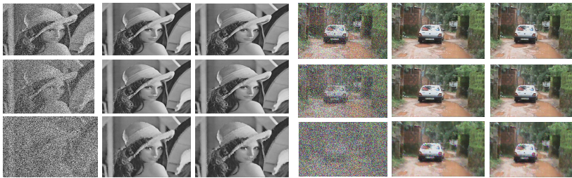
Fig. 4. Results of proposed Method for Gray Scale Lena Image and Car Image (a) Images Corrupted with 20%,50% and 80% Salt and Pepper Noise (b) Noise Reduced by Improved Median Filter (c) Enhanced Images Using Morphological Operation
