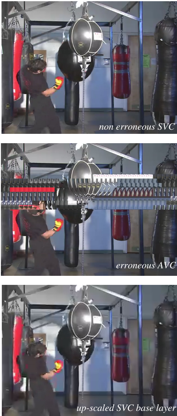
Fig. 3. Overview of the distortions introduced by coding artifacts, conventional error concealment techniques and spatial up-scaling
