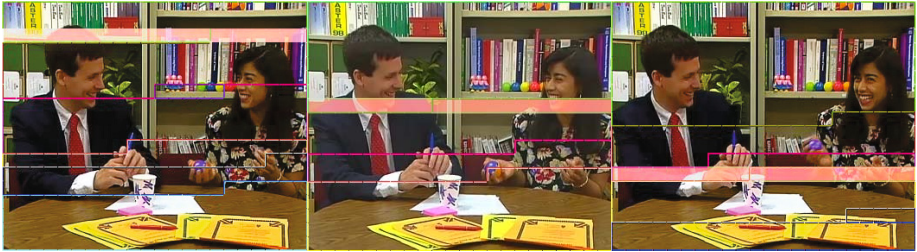
Fig. 2. Cyclic intra-refresh MB line technique for the Paris test sequence, showing successive MB lines in lighter shading, with some slice boundaries also shown
