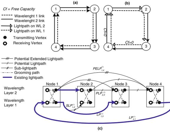
**Fig. 5.** (a) An example of a four-node network with two wavelengths in each fiber; (b) the current state of the network with available wavelength links; (c) the auxiliary graph,  $GG$ , for the current state of the network shown in (b).
