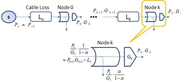
**Fig. 3.** Power budget model for supporting lightpath extension and lightpath dropping using TOP-enabled node architecture
