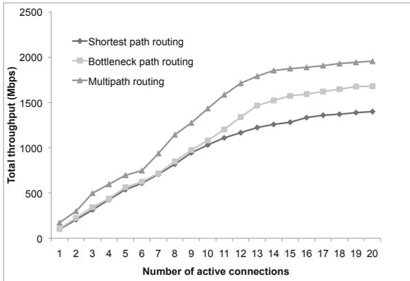
**Fig. 3.** Network saturation as the number of active connections increases
