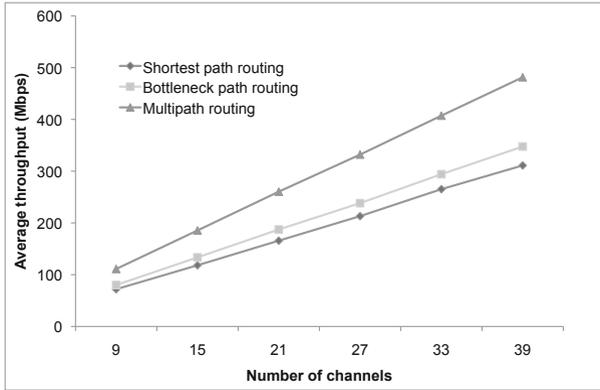
Fig. 2. Average path transmission rate versus the number of available channels
