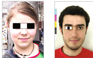
Fig. 9. Application of two sample rectangular features for face and eye detection
