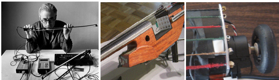
Fig. 5. left to right, Jon Rose with his MIDI Bow, CNMAT’s augmented cello for Francis-Marie Uitti and a close-up of its wheel encoder (driven by the bow)
