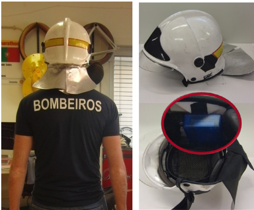
Fig. 3. The new VR Vital Jacket for firefighters had to comply with both international safety regulations for textiles under high heat conditions and the Portuguese law on firefighter garments. As a result, the new shirt (left) visually mimics the normal shirt worn by firefighters and now has less than 2% elastane. Temperature, barometric pressure and carbon monoxide sensors were also embedded in a firefighter helmet model that complies with all EU safety regulations (right).
