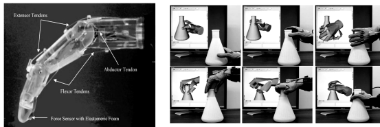
Fig. 6. Left : An artificial finger, [10]. Right : Examples of interactive grasp planning using input provided by an operator, [11].
