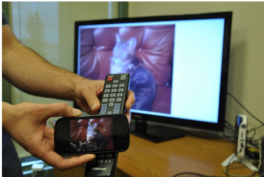
Fig. 4. Pushing multimedia to a remote display after touching a phone to a TV remote control
