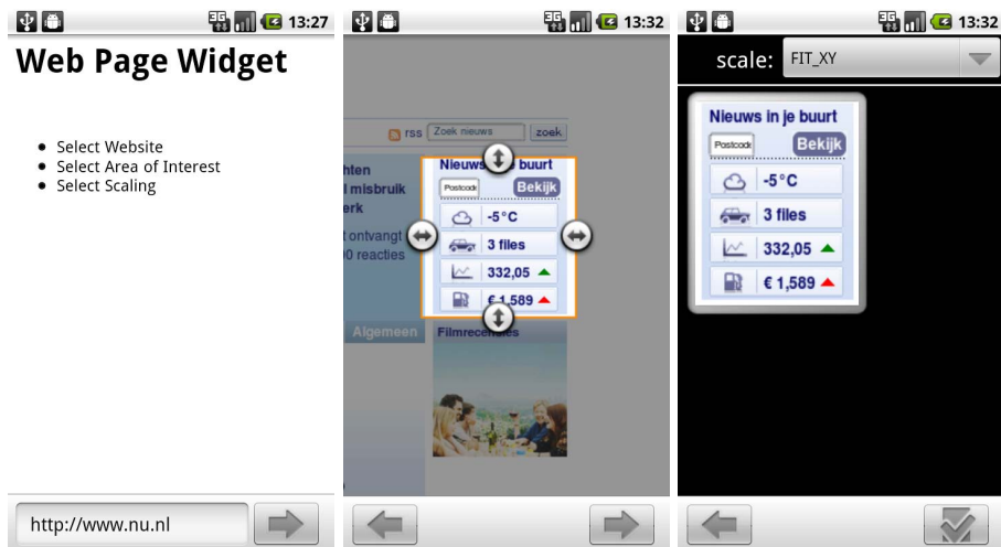
Fig. 8. Configuration of a Web Page Widget. First a URL of a to be monitored website is entered. Then this webpage gets rendered at the remote resource an image is sent back to the phone. The user now selects the area of interest. Finally, the user can specify how the image will be mapped onto the area on the screen.
