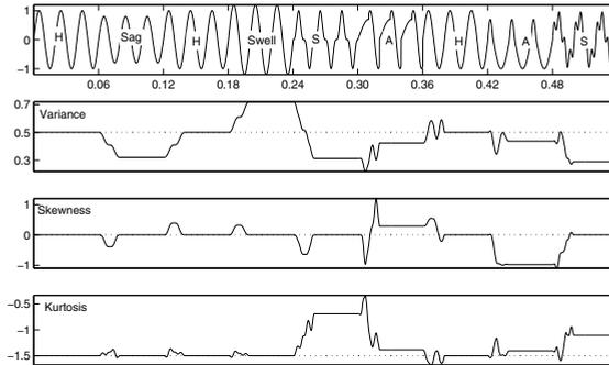
**Fig. 2.** On site measurement simulation which shows the evolution of the constant values associated to three statistics (variance, skewness and kurtosis)
