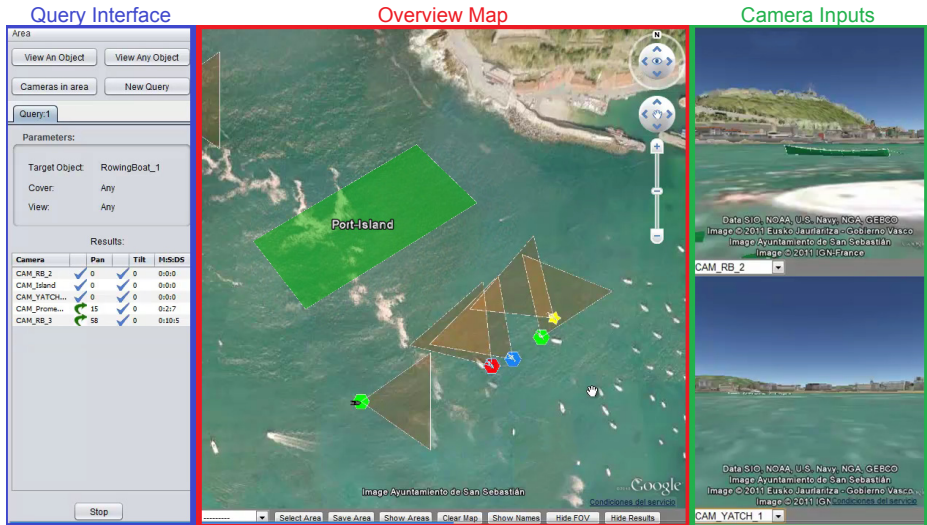
Fig. 1. Graphical User Interface using Google Earth plugins to simulate cameras
