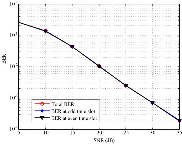
Fig. 6. The BER of FRAF with precoding
