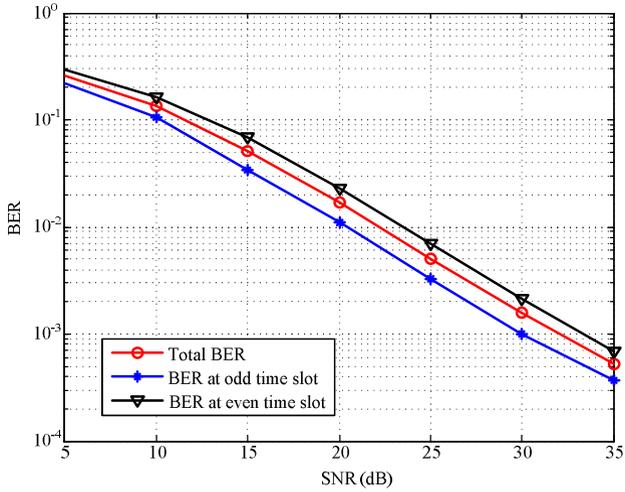
Fig. 5. The BER of FRAF without precoding
