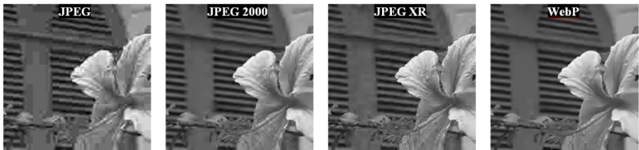
Fig. 7. Portion of image 7 (from the Kodak dataset) compressed at 0.26 bpp
