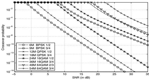
**Fig. 3.** Crossover probability vs. SNR, Rayleigh channel
