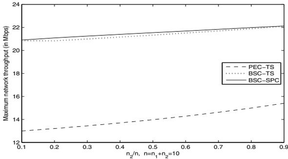
**Fig. 9.** Unicast maximum network throughput vs. varying proportion of class 2 stations for a fixed total number of stations  $n_1 + n_2 = 10$ ,  $SNR = 22\text{dB}$ ,  $L = 8000$  bytes, Rayleigh channel
