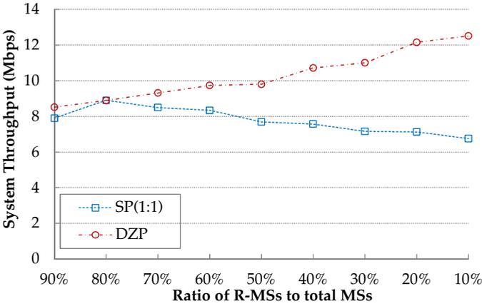
Fig. 2. System throughput for various R-MSs to total MSs ratios
