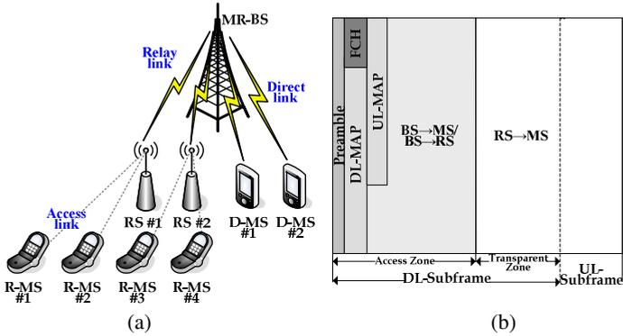
Fig. 1. IEEE 802.16j transparent relay networks: (a) topology and (b) frame structure
