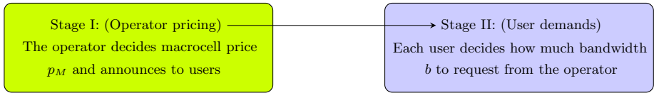
Fig. 1. Two-stage Stackelberg game between the operator and users. Stage I: the operator decides macrocell price per unit bandwidth to maximize its profit. Stage II: users choose how much resource to request in order to maximize their payoffs.
