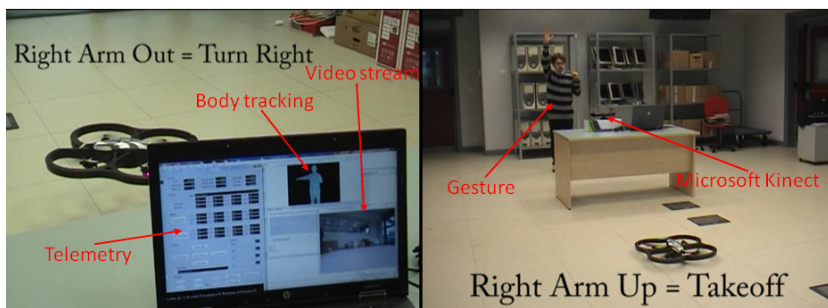
Fig. 4. Two pictures of the experimental setup. On the left the laptop console is shown, whereas the Microsoft Kinect is visible on the right.
