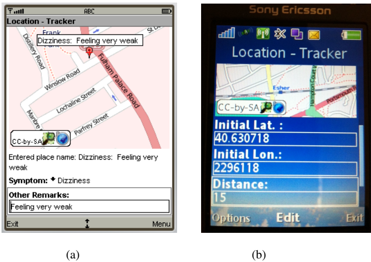
Fig. 2. (a) Sample reactive, location-based service: reporting a health symptom on a map, and (b) sample proactive location-based service: tracking the location of a person with Alzheimer's disease
