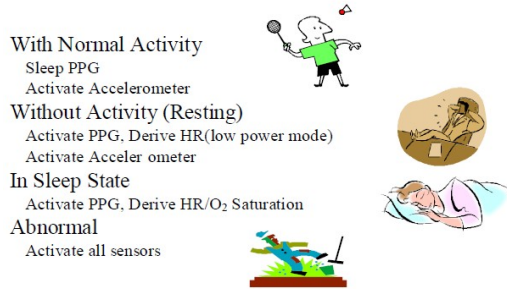
Fig. 2. Operation modes of hybrid vital sensor
