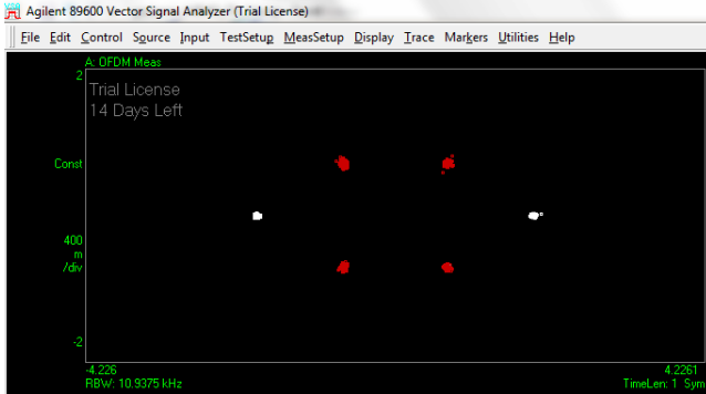
Fig. 2. Demodulation of the MIMO signal transmitted by CTTC’s real-time FPGA-based MIMO-OFDM mobile WiMAX transmitter, using Agilent’s VSA signal analysis software
