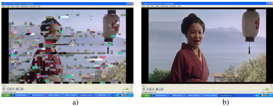
Fig. 5. Perceptual illustration of the smart antenna benefits. Received movie snapshot for: a) omnidirectional antenna. b) smart antenna.
