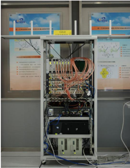
**Fig. 6.** Installation of the Gbps Wireless Testbed (one side)
