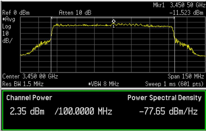
(a) Output Signal at a Transmitter Antenna
