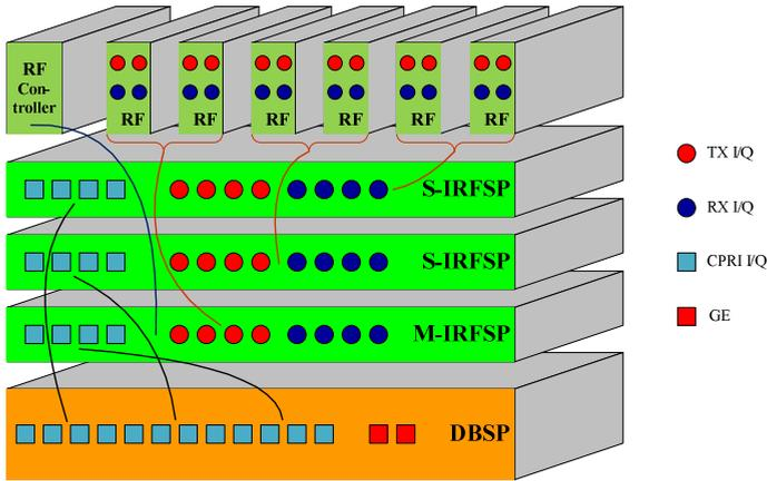
Fig. 1. System Architecture of Hardware Platform
