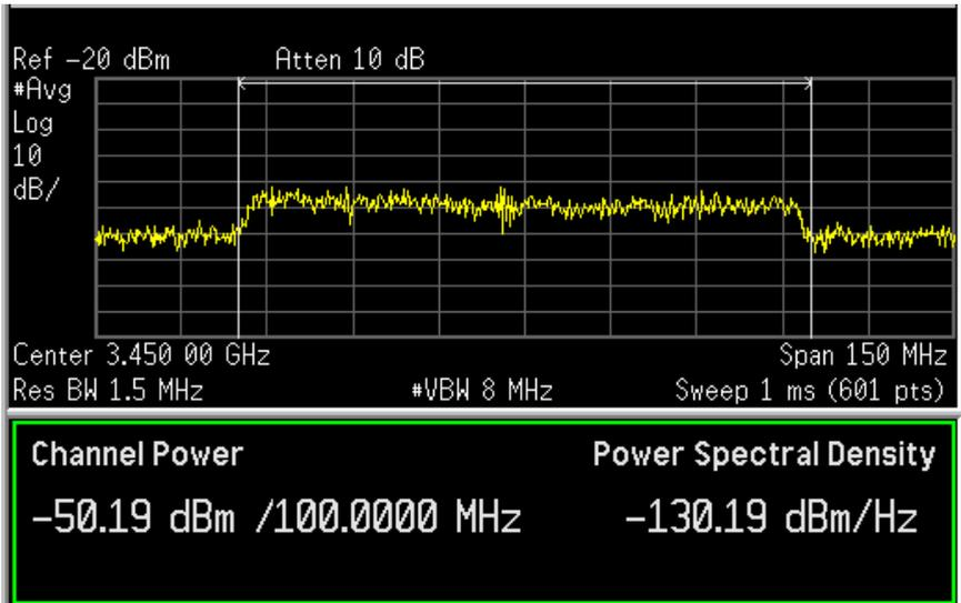
(b) Input Signal at a Receiver Antenna
