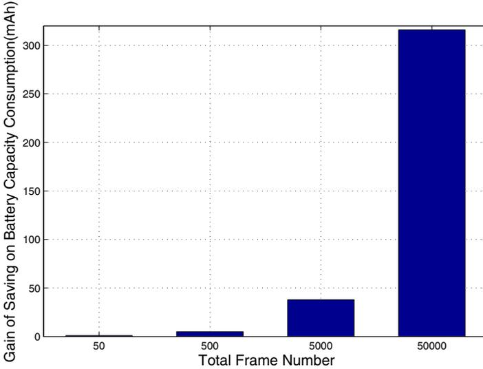
**Fig. 8.** Comparison of battery capacity saving in delivering 50, 500, 5000 and 50000 frames
