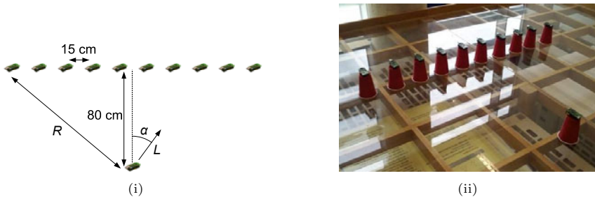
Fig. 1. Experiments for testing multiple sensors' RSS. (i) \alpha denotes the angle between the receiver's moving direction and the perpendicular bisector of the transmitters. R is the sensor's communication range, which is about one meter. (ii) Experimental setup.
