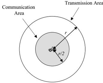
Fig. 1. Transmission area and communication area
