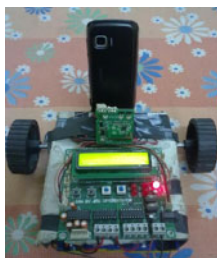
Fig. 3. Robot prototype consisting of microcontroller, CC2500 module and Bluetooth enabled camera
