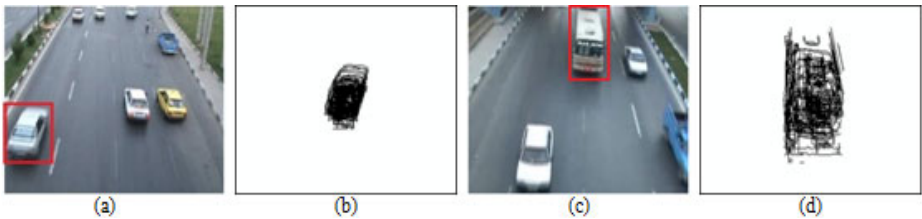
Fig. 2. (a) A sample car enclosed in a bounding box. (b) The shifted boundary curves of the car to the center of a framework during its tracking. (c) A sample bus circumscribed by a bounding box. (d) The located boundary curves of the bus to the center of a framework while it is tracking.
